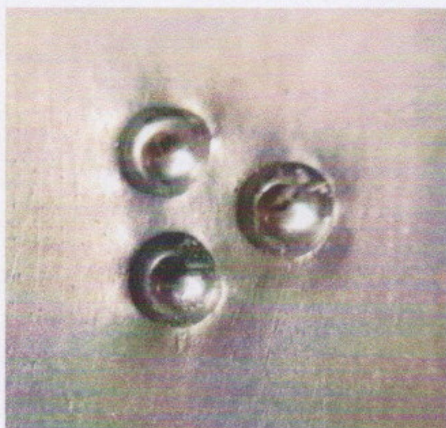
Figure 4 - Indentations of the 1 rod welded sample
