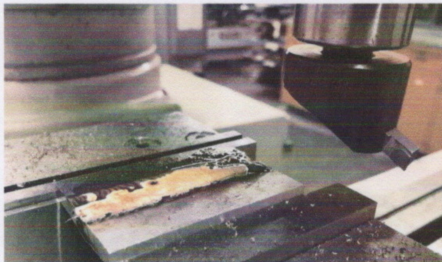
A3 - Carbide fly cutter used to remove weld reinforcement
